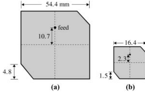
**FIGURE 1.1** Circularly polarized corner-truncated square microstrip antennas for GPS application at 1575 MHz. (a) Design with a microwave substrate ( $\epsilon_r = 3.0$ ,  $h = 1.524$  mm); (b) design with a ceramic substrate ( $\epsilon_r = 28.2$ ,  $h = 4.75$  mm). Dimensions are in millimeters and not to scale.
