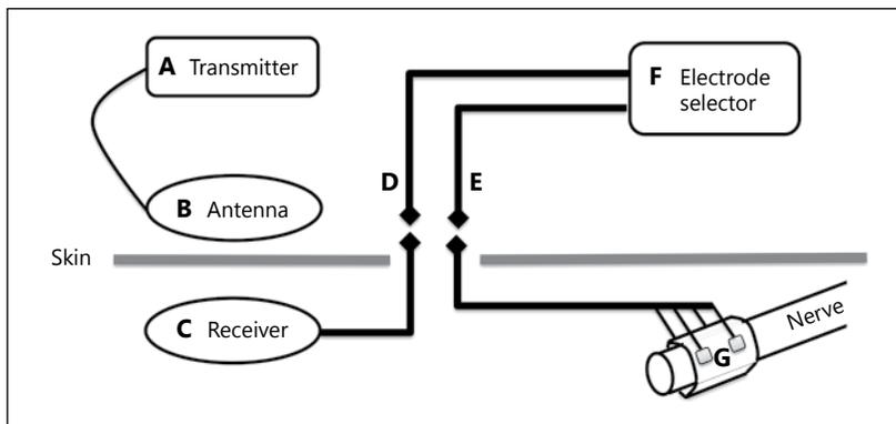
**Fig. 3.** Schematic representation of the components of the Avery PNS system. Before internalization of the lead, the electrodes (**G**) are connected by wires (**E**) and connectors (**D**) to the electrode selector (**F**); when the optimal electrodes are determined, they are connected to the internal receiver (**C**). Stimulation is transmitted to the receiver (**C**) via an antenna (**B**) attached to the transmitter (**A**).
